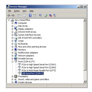
Figure 47. Device Manager Virtual COM Ports
