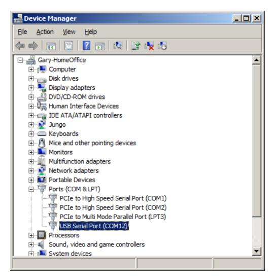
Figure 24. Device Manager and COM Port Assignments
