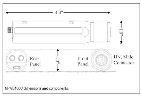
Figure 5. NPM3100U Device Dimensions
