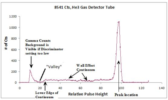
Figure 43: Typical He3 Histogram (Pulse Ht Spectrum)
