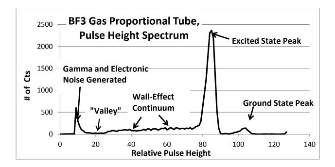
Figure 44: Typical BF3 Histogram (Pulse Height Spectrum)
