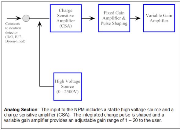
Figure 2. Analog Section.
