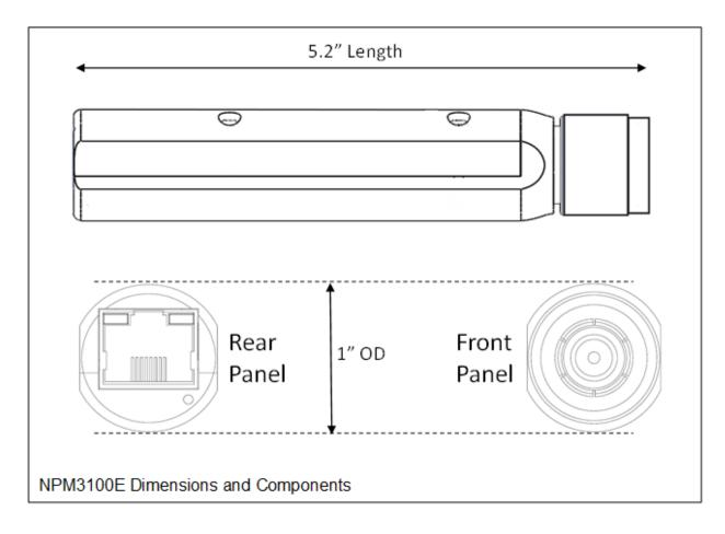
Figure 7. NPM3100E Device Dimensions.
