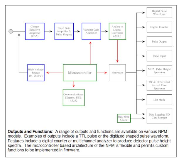
Figure 4. Outputs and Functions.
