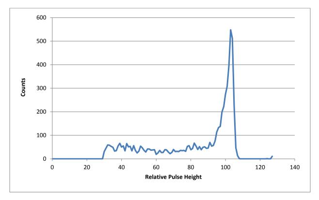
Figure 21. Helium-3 Detector HGM (Pulse Height Spectrum)
