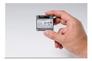
The latest generation Iridium SBD modem are small, lightweight, and consume low amounts of power. This modem is utilized in Quaesta Instruments Iridium enabled dataloggers, such as the Q-DL-2100-I.
